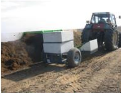
Processing equipment: Tractor-pulled turner and final product screening
