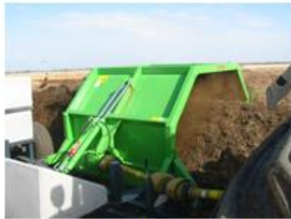
Processing equipment: Tractor-pulled turner and final product screening
